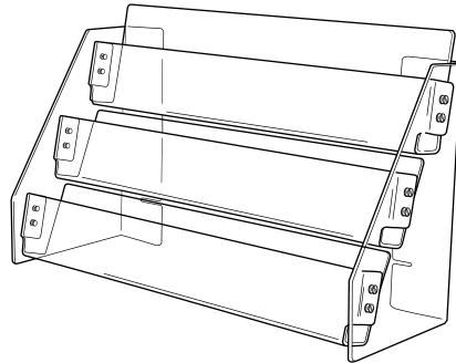
4, Attach the top and bottom shelves. Once the shelves are attached, check for proper positioning and square and gently tighten all screws.
