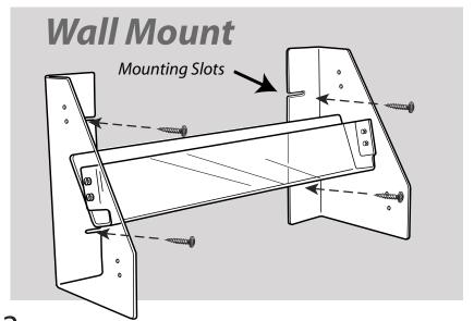
**3, For wall mount:** If you are mounting on a wall, now is the time to attach the rack to the wall. Place mollie bolts (or wood screws with screw anchors through the slots in the back plate.
