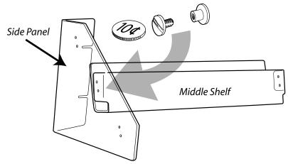
2, On a clean flat surface, attach the center shelf to each side panel with the binding post screws.
