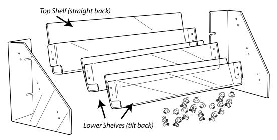
1, Carefully unpack and identify all parts. 2 side panels, one top shelf, two lower shelves, and 4 binding post screws per shelf.
