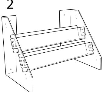
four shelves, and 4 binding post screws and nuts per shelf. Note that the tall side of each shelf faces to the back of the unit.
