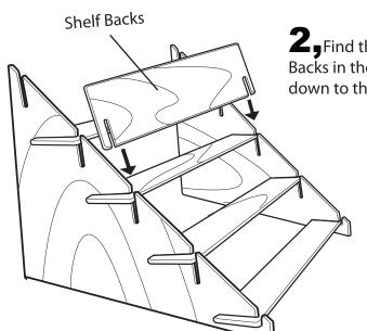
**2** Find the 4 *Shelf Backs*. Insert the Shelf Backs in the vertical slots by pressing them down to the bottom of the slots.
