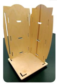
Insert regular side panel into the first side panel's slot and fit the bottom onto the base.
