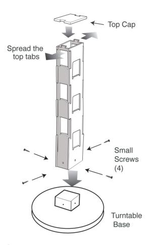
4. Attach the Tower Assembly to the Turntable Base using the 4 small screws.
