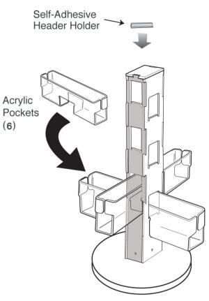
**6.** Starting from the base, slide the Acrylic Pockets into the holes and press down to lock them in place. on top.
