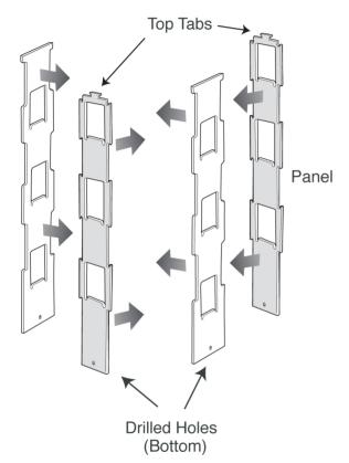
2. Position tabbed and slotted panels as shown. Note the two different pairs of panels go on opposite sides. Gently press tabs into slots and wiggle and flex the tabbed panels to lock them in place.
