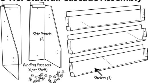
1, Locate and Identify all parts: 3 shelves, 2 side panels, and 12 binding screw and nut sets.
